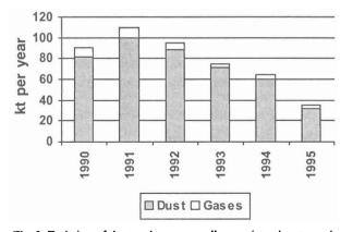
Fig. 2. Emission of dust and gaseous pollutants into the atmosphere from the cement plant in Kunda in 1990-95
